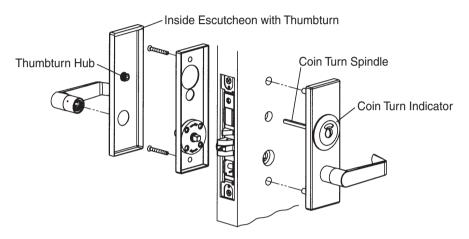
III. In case emergent situation, use a coin or flap tip screwdriver to unlock door.
