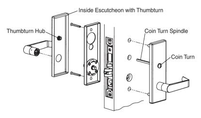
III. In case emergent situation, use a coin or flat tip screwdriver to unlock door.
