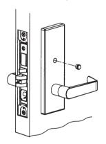
II. In case emergent situation, remove this outside emergency release cap, and insert a Phillips screwdriver into the thumbturn hole and rotate it to unlock door.
