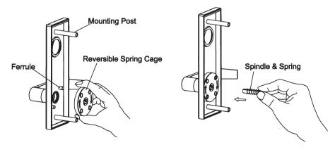
C.Install outside lever with mounting posts through door and position spindle with spring into hub of lock case.
